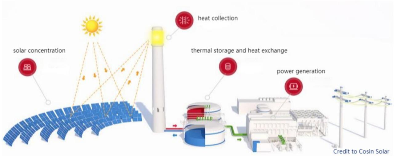
Figure: molten salt solar tower plant diagram
