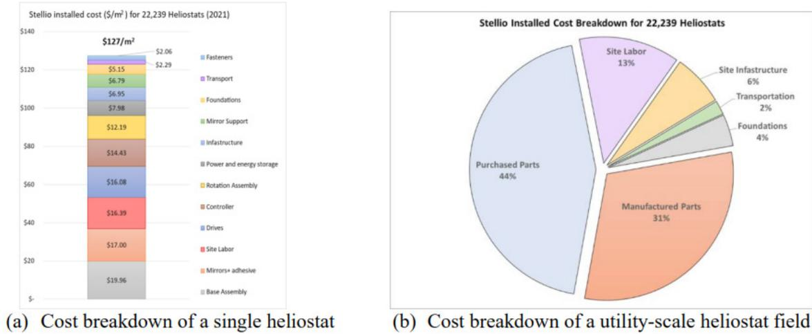
Figure: sbp Stellio heliostat cost breakdown (Source: Roadmap to Advance Heliostat Technologies for Concentrating Solar-Thermal Power, 2022 Heliocon)
