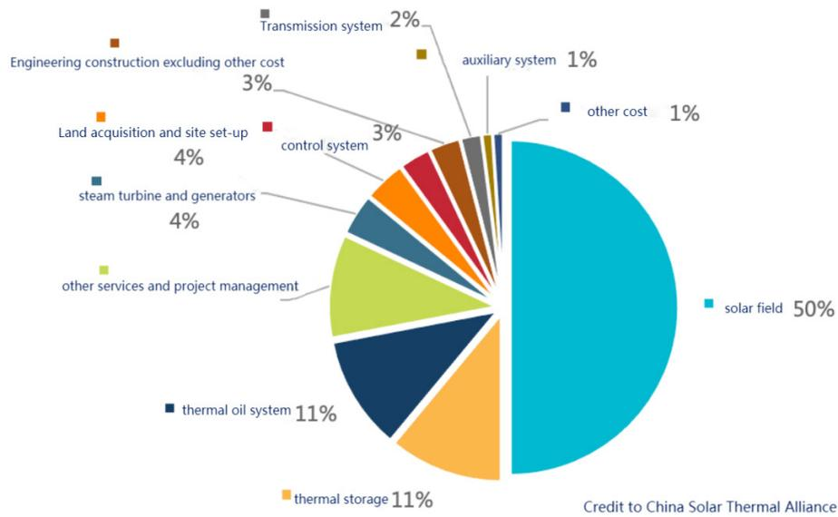
Figure: Investment composition of China's a 50MW parabolic trough plant with 4h thermal storage system
