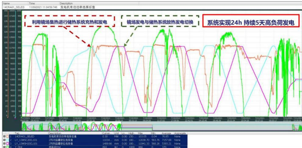
Figure: From July 17 to 21 2021, the power station realized 24h/5 consecutive days of high load power generation
