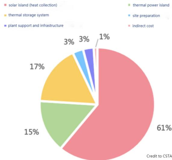
Figure: Investment composition of 50MW solar tower power plant with 7-hour thermal storage
