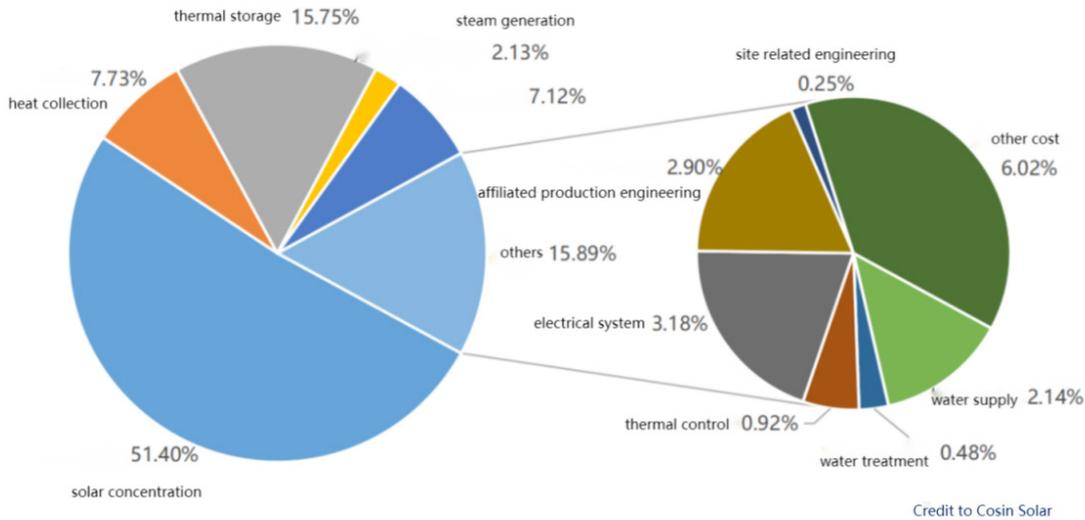
Figure: Investment composition of a 100MW solar power tower plant with 12h thermal storage system
