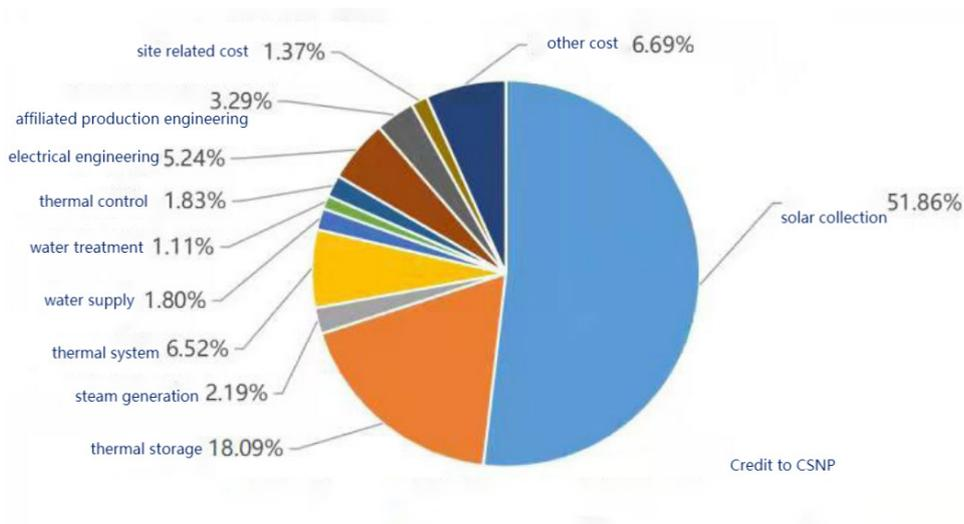
Figure: Investment composition of one 100MW parabolic trough power plant with 10h thermal storage system
