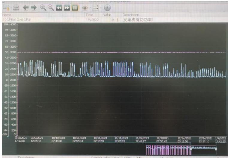
Figure: Steam turbine speed and load curve chart of CGN Delingha 50MW Parabolic Trough Power Plant
