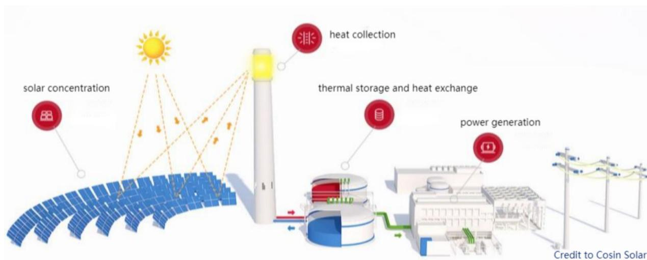
Figure: molten salt solar tower plant diagram
